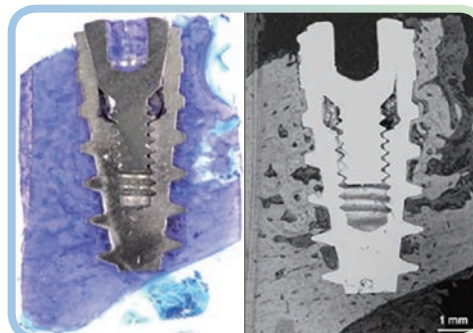
Fig. A The histological cross-section of the Azure C-System Implant with new bone formation.
